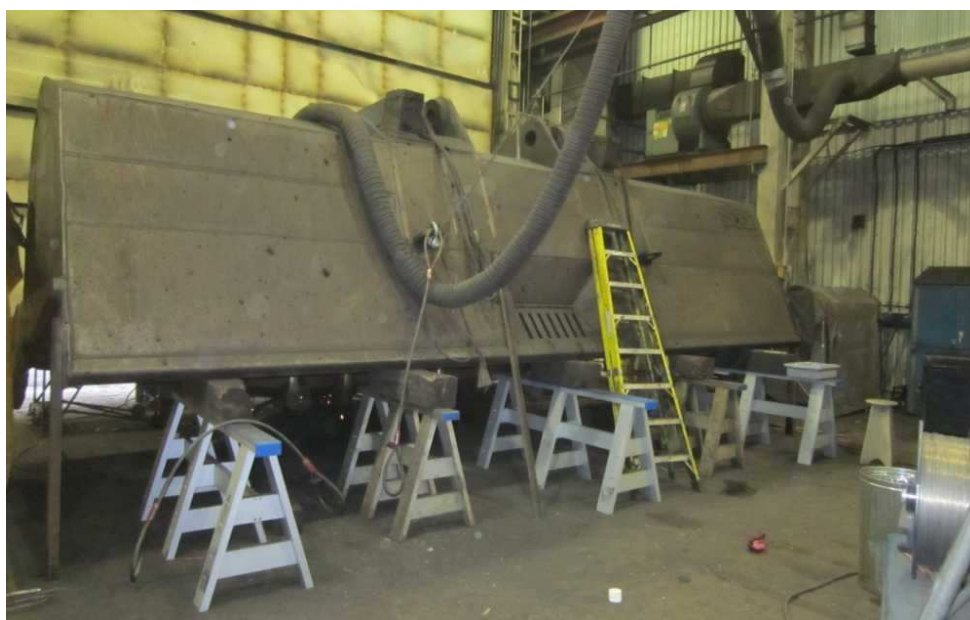
Five HBTC saw horses safely supporting a front-end loader bucket, weighing 43,000 lbs.
